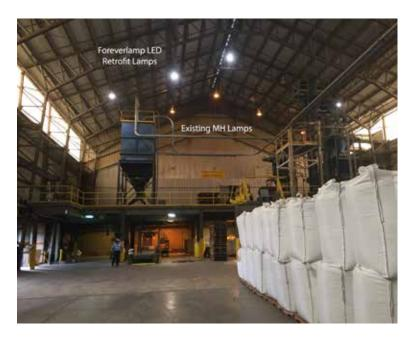
equivalent solution could serve the needs ideally with a downlight or uplight / downlight option. For higher ceilings of 35ft and above, a 1000W solution should be considered.
