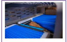
With the multi-aperture, multi-lane metal detector, each lane works independently, enabling a potential contaminant to be isolated without rejecting good product from other lanes.
