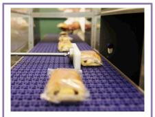
False rejects occur when good product is identified as containing a metal contaminant and can cost a food manufacturer up to \$14k annually per line.
