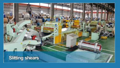
Slitting shears is widely used for longitudinal shear thickness less than 20-30mm steel and thin strip. Because the blade is rotating disk, which can cut a moving continuous longitudinal steel or steel.
