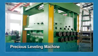
The machine adopts pneumatic clamp connection dovetail clamping plate, clamp easy to move, reduce the bending deformation of the material, reducing processing dead zone, a large selection of high-precision servo motor torque, long life, high precision drive, through the machine after leveling can be corrected material to bend up and down or flat.
