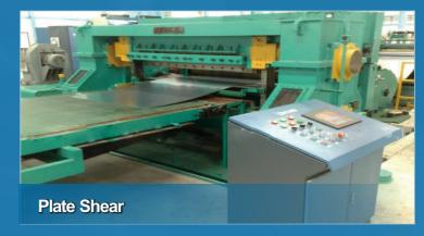
Shears with a blade relative to the other reciprocating linear motion of the shear blade for sheet metal machine. Is in motion by the blade and the fixed lower blade, using reasonable blade clearance, applying a shearing force on the sheet metal of various thicknesses, the sheet material separated by the desired size of the fracture.
