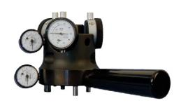
Using the taper shank test fixture, JMPP redesigned the knobs, finally reaching a design that eliminated or substantially eliminated toolholder expansion. Their patented High Torque retention knobs are designed to thread deeper into the bore of the holder where there is a thicker cross-section of material to resist deformation.
