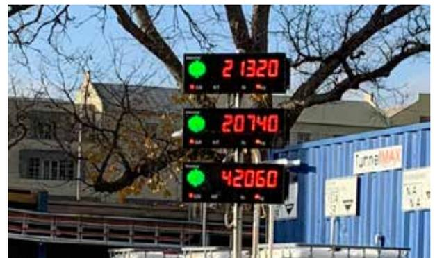
LED displays allow the driver to view live axle weights to keep from leaving the worksite overloaded, or causing inefficiencies due to an under-loaded truck.
