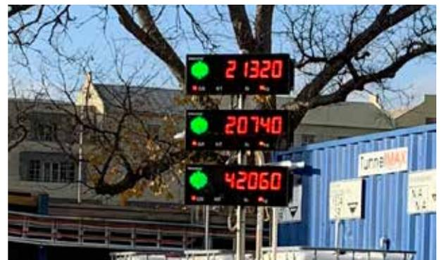
LED displays allow the driver to view live axle weights to keep from leaving the worksite overloaded, or causing inefficiencies due to an under-loaded truck.
