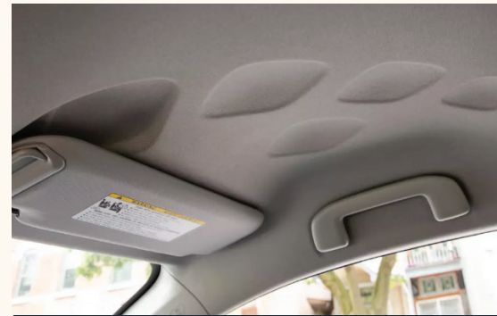
A headliner is the material that covers the ceiling of a vehicle, but it does more than hide bare metal with color-coordinated soft fabric.
